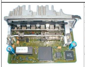
CENTRALINA DI GESTIONE MOTORE MA1.3 INSTALLATA SULLE VETTURE DEL GRUPPO VAG BENZINA.
